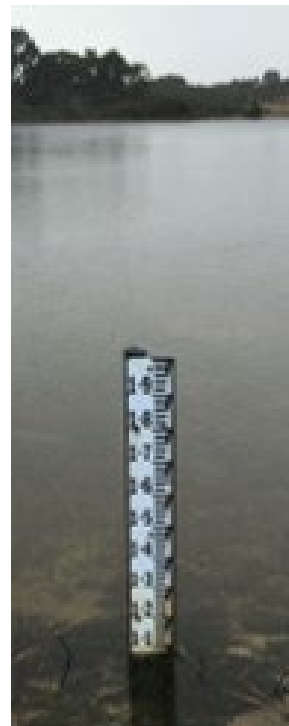
Figure 1. Simple stilling well and Staff Gauge Setup (DRW, 2016).
