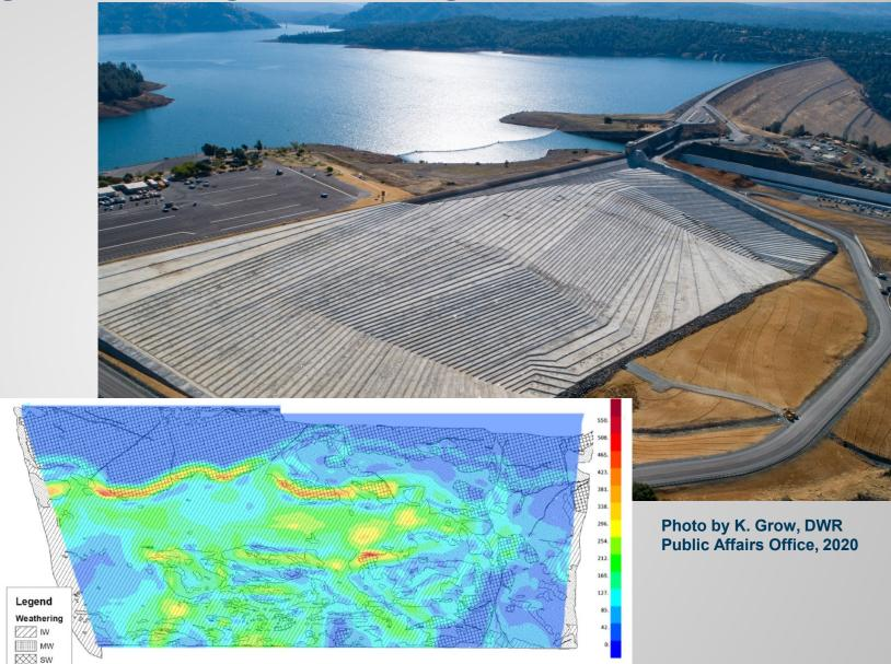
Figure 21 – von Mises Stress (ksi) due to Self-Weight overlain on Revised RCC Apron Geologic
