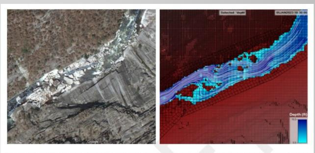
Figure 34. An example of flood depth overlaid with the velocity streamlines from the 2D HEC-RAS model at a rocky section of the MF Feather River for the 5-year event.
