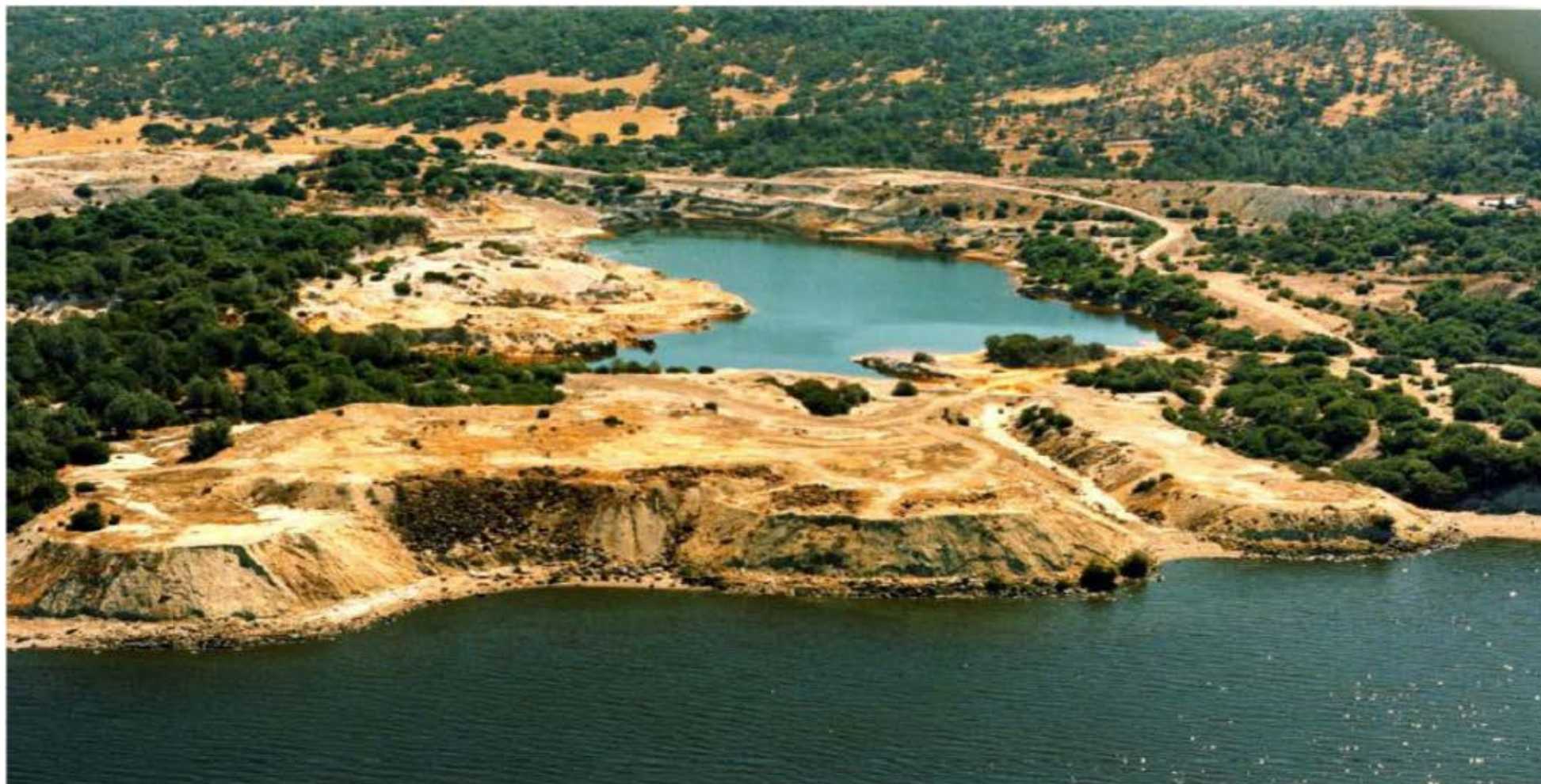
PLATE 8. Sulphur Bank Mercury Mine showing steeply sloped waste rock piles that comprise the waste rock dam with overflow channel into Clear Lake (on right side of dam) before the 1992 slope remediation by U.S. EPA. Note 30 m deep Herman Pit (pH~3) in background. Clear Lake is in the foreground. (Courtesy of Charles Chamberlin, Humboldt State University; photo taken in 1987, before waste rock pile remediation in 1992).
