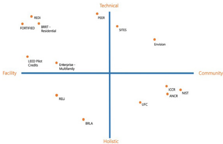
Figure 7.5: Voluntary standards in the building sector fall into a number of categories, here classified by whether they are technical or more holistic in focus, and whether they focus on a single facility or a community (Source: Meister Consultants Group 2017 [254] , used with permission)
