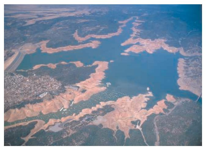
Lake Oroville in 1990. Oroville Dam is at left edge of photo. The 3.54 maf reservoir was at about one-third capacity at the time of this photo. During the 1976-77 drought, its storage declined to about one-quarter of full capacity.
