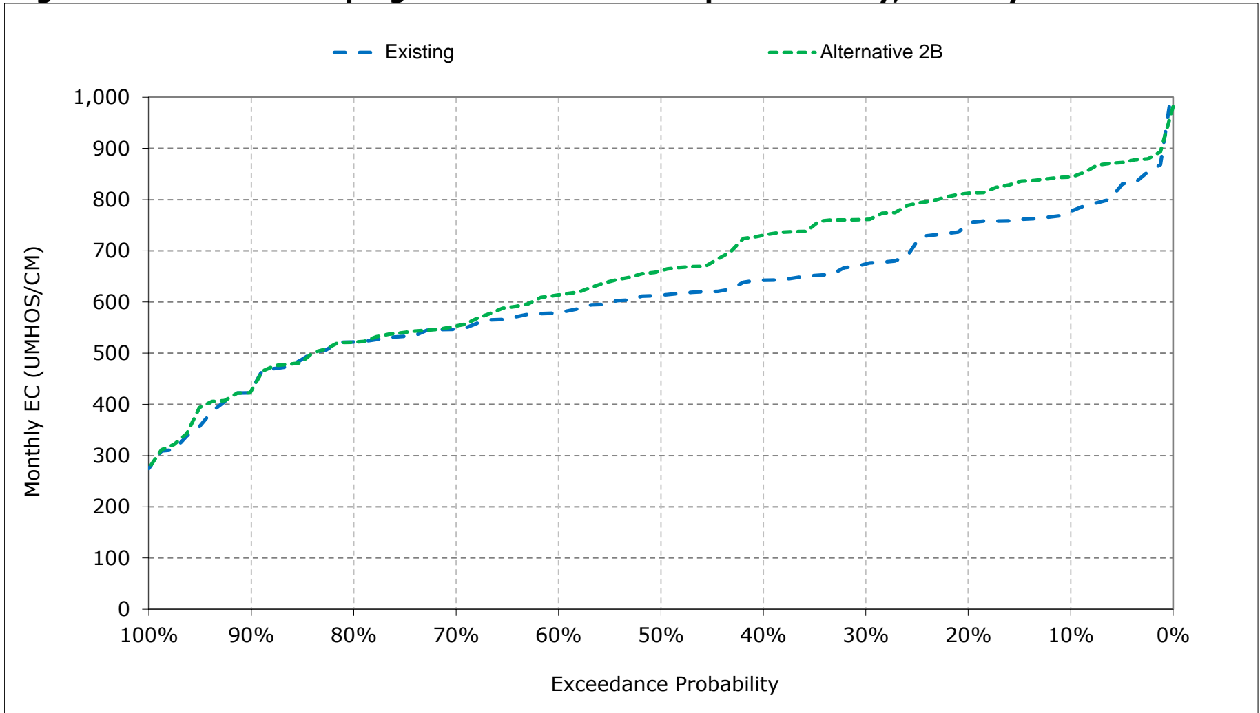
Figure 17-7. Jones Pumping Plant South Delta Exports Salinity, January EC
