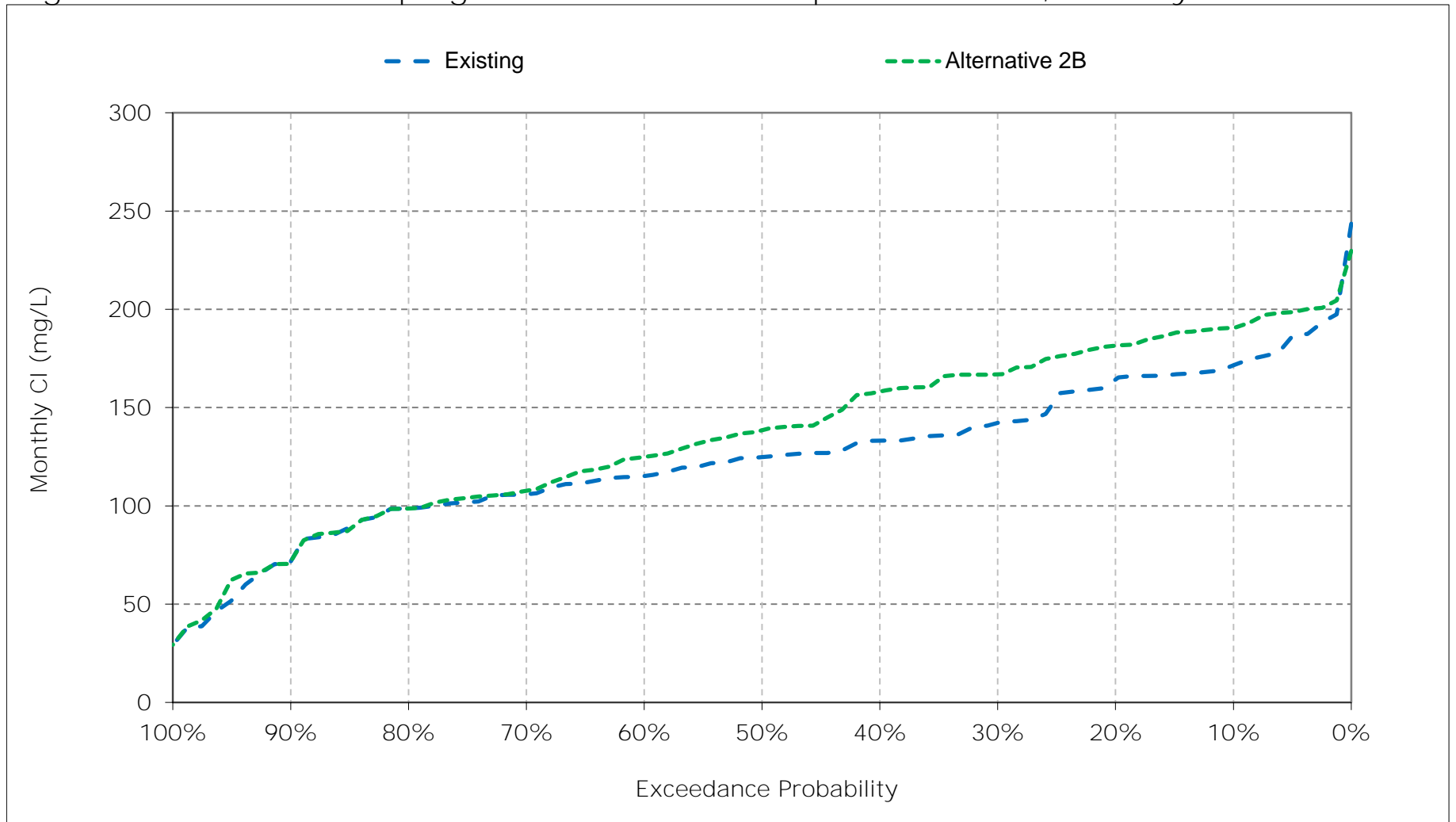
Figure 12-7. Jones Pumping Plant South Delta Exports Chloride, January CI
