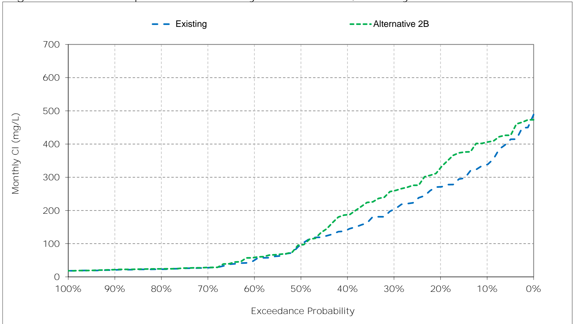
Figure 4-7. San Joaquin River at Jersey Point Chloride, January CI
