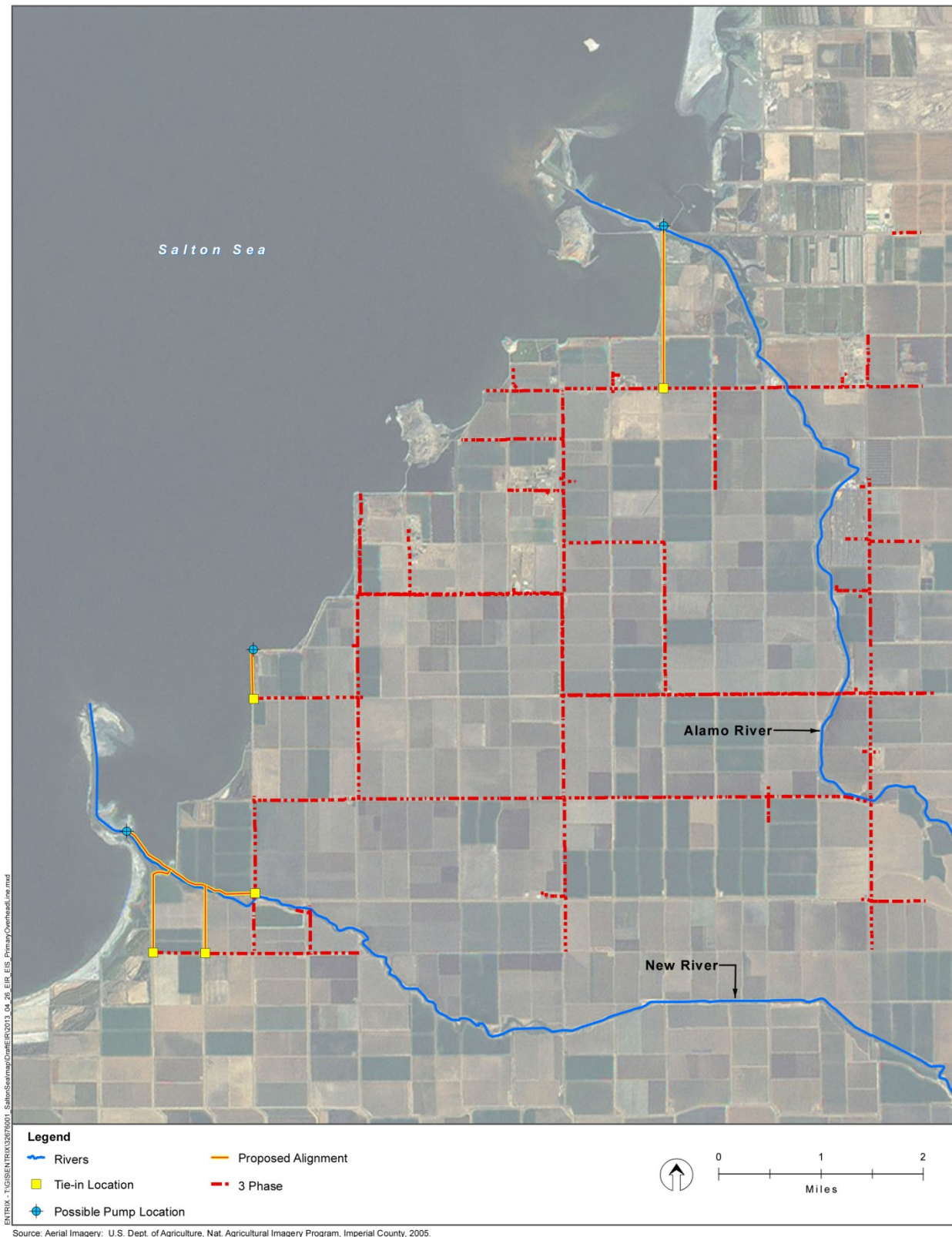
Figure 2-5 Location of IID's Three-Phase Power Lines and Potential Project Extensions
