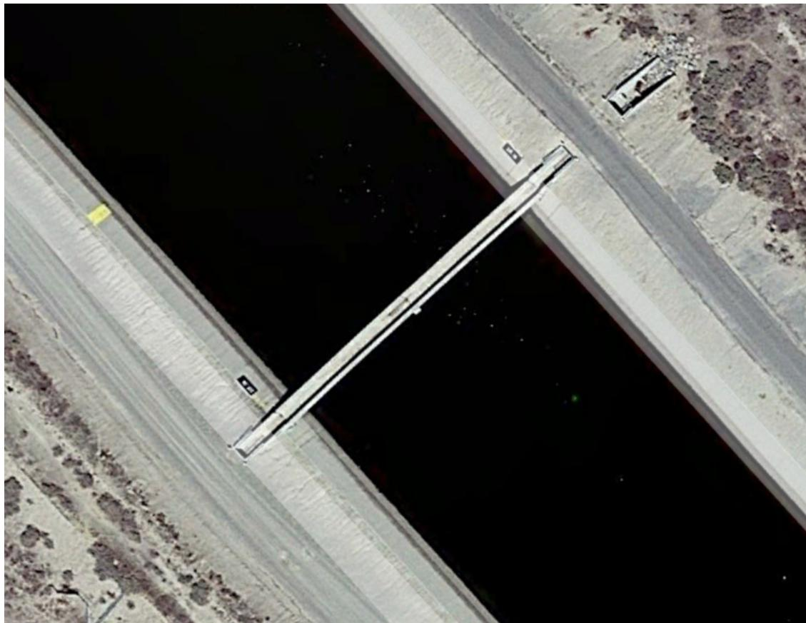
**Figure 2-4. Aqueduct Overchute Near MP 235.07**
