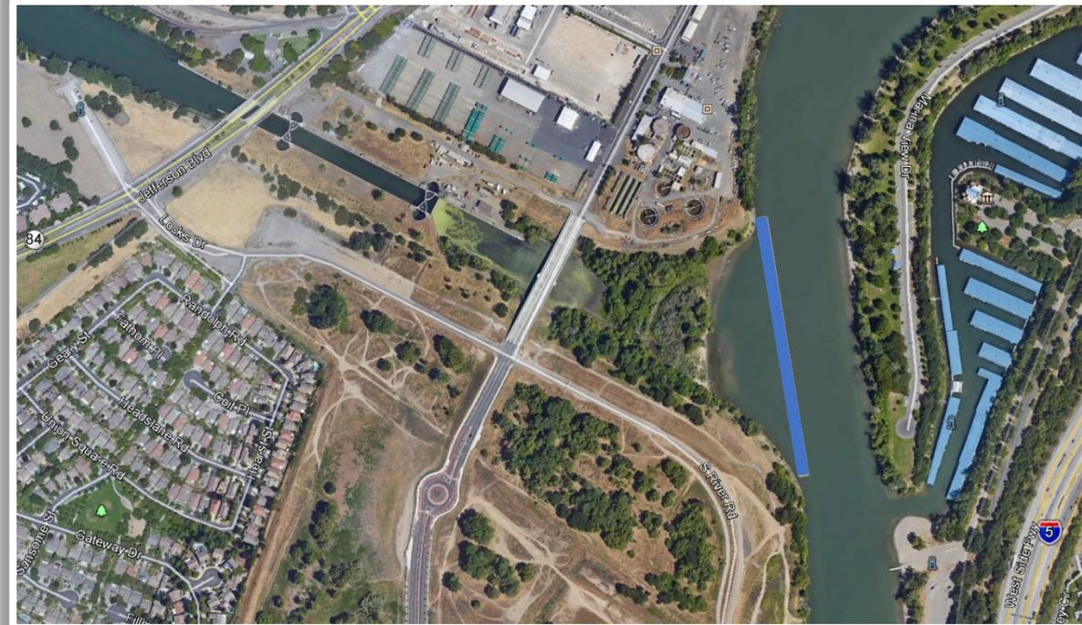
Approximate length of 3,000 cfs flat plate fish screen at confluence of Ship Channel and Sacramento River using actual river bathymetry data.
