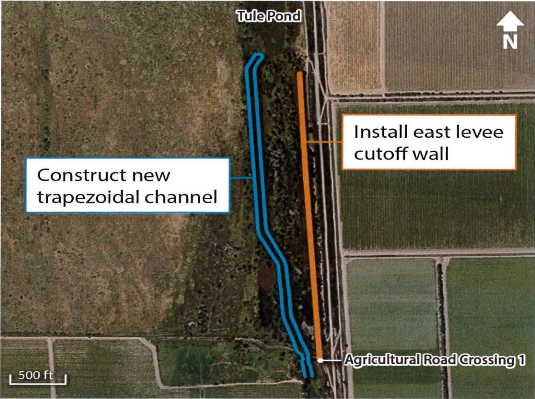
Figure 4. Downstream improvements near Agricultural Road Crossing 1
