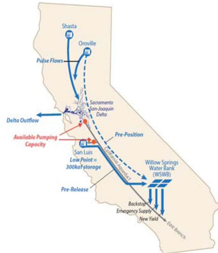
Figure 1 - Schematic of Willow Springs Water Bank Conjunctive Use Project
