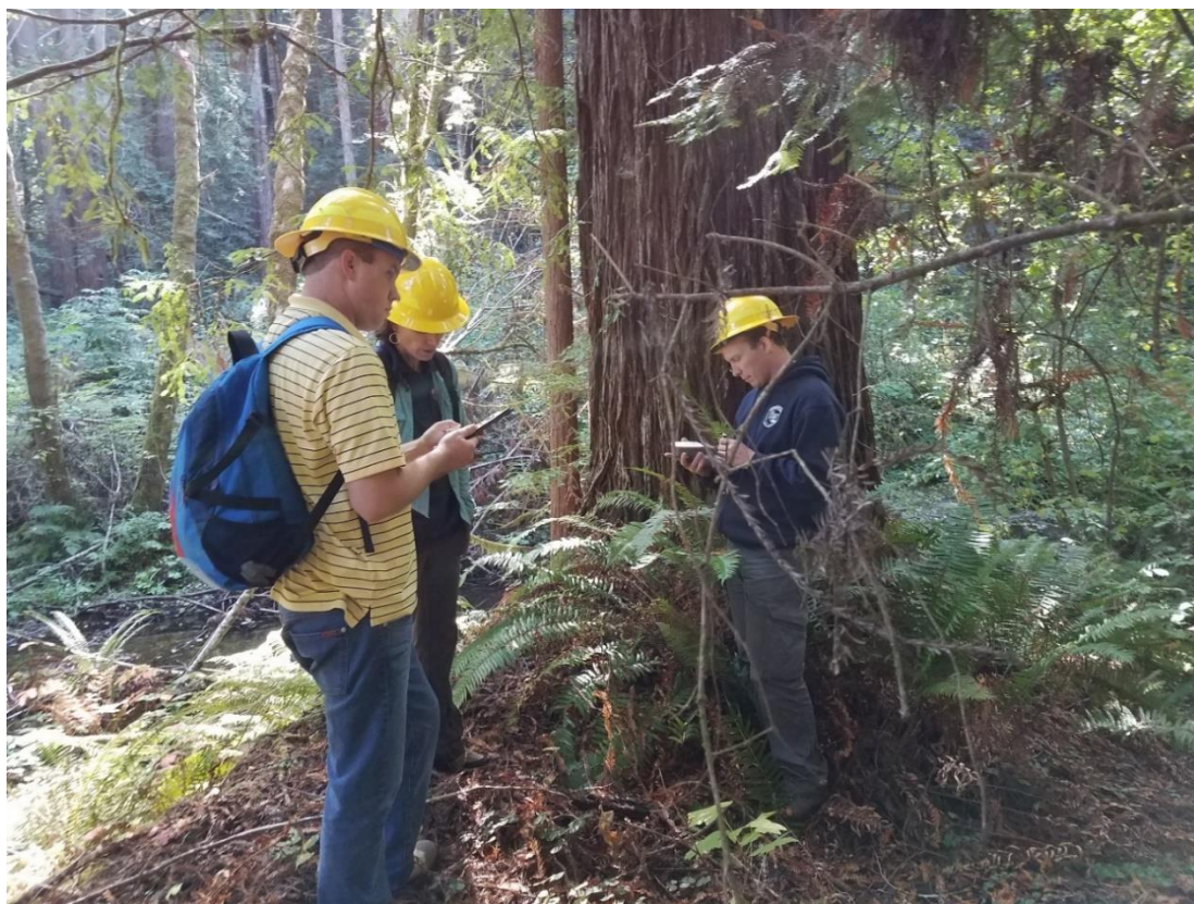
Figure 21. Field team in the Smith Creek planning watershed on October 10, 2018 comparing measured tree heights to LiDAR derived tree heights.
