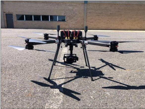
Photograph of the BFD Systems SE8 Unmanned Aerial Vehicle.
