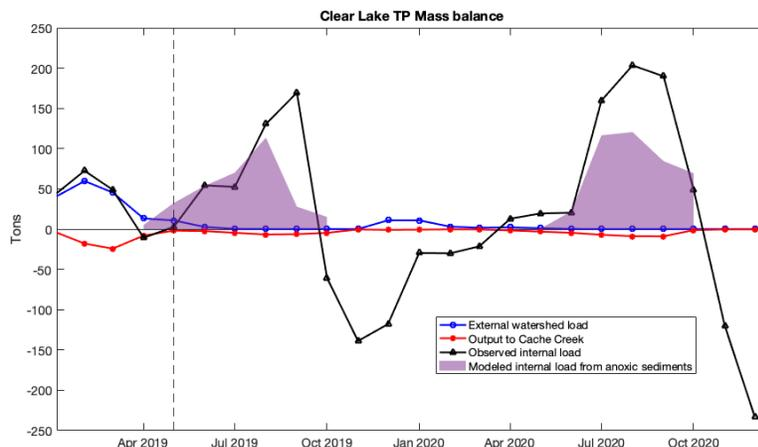
Figure 1 – Total phosphorus mass balance for Clear Lake (2019-2020). Dashed vertical line indicates the start of the UC Davis Lake monitoring program.
