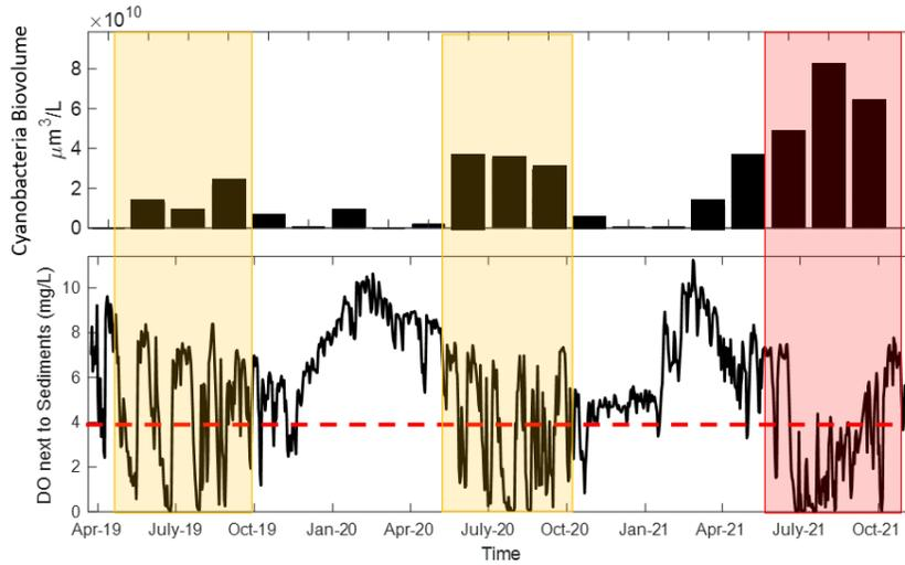
**Fig. 1.** (Top) Cyanobacteria biovolume from our in-lake sampling every 6-8 weeks in the Oaks Arm. (Bottom) Continuous-time series of benthic dissolved oxygen in the Oaks Arm. The red dashed line marks one of the possible DO thresholds to define hypoxia. The squares mark the summer periods when the cyanobacteria biovolume increases and the DO decreases
