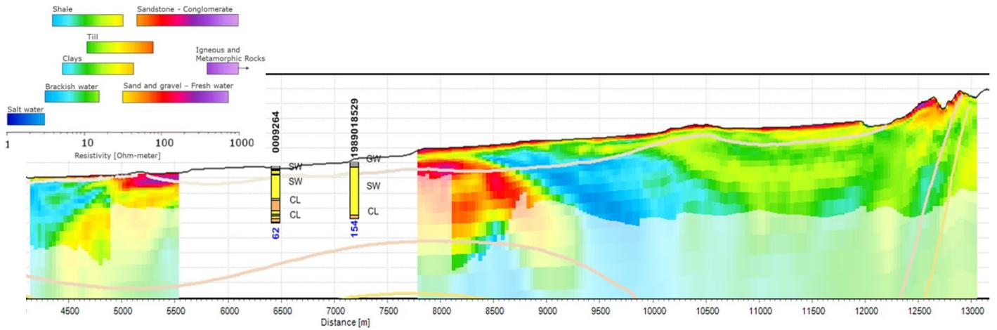
Figure 2 (AEM interpretation of a slice through the subsurface and well logs to fill data gaps)
