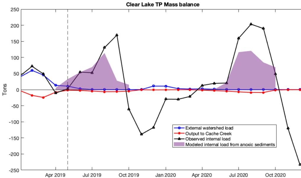
**Fig.2.** Total phosphorus mass balance for Clear Lake (2019-2020) with external input and output loads, and observed and modeled internal load from anoxic sediments using laboratory P-release rates. Dashed vertical line indicates the start of the UC Davis Lake monitoring program
