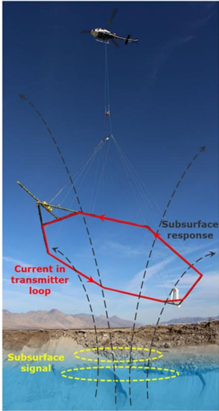
Figure 1 (AEM geophysical instrument breakdown)
