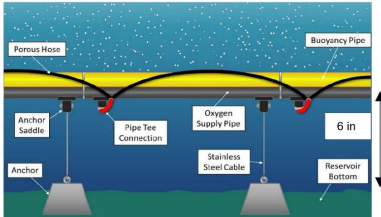
**Fig. 5.** Oxygen diffusers diagram. The yellow pipeline is very porous and it releases fine bubbles creating a crater that removes the sediments that may be covering it. The black pipe transports the oxygen and it is designed to float and keep the diffuser above the sediments
