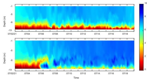
Fig. 8. Three-dimensional lake model results of dissolved oxygen without hypolimnetic oxygenation (top) and with
