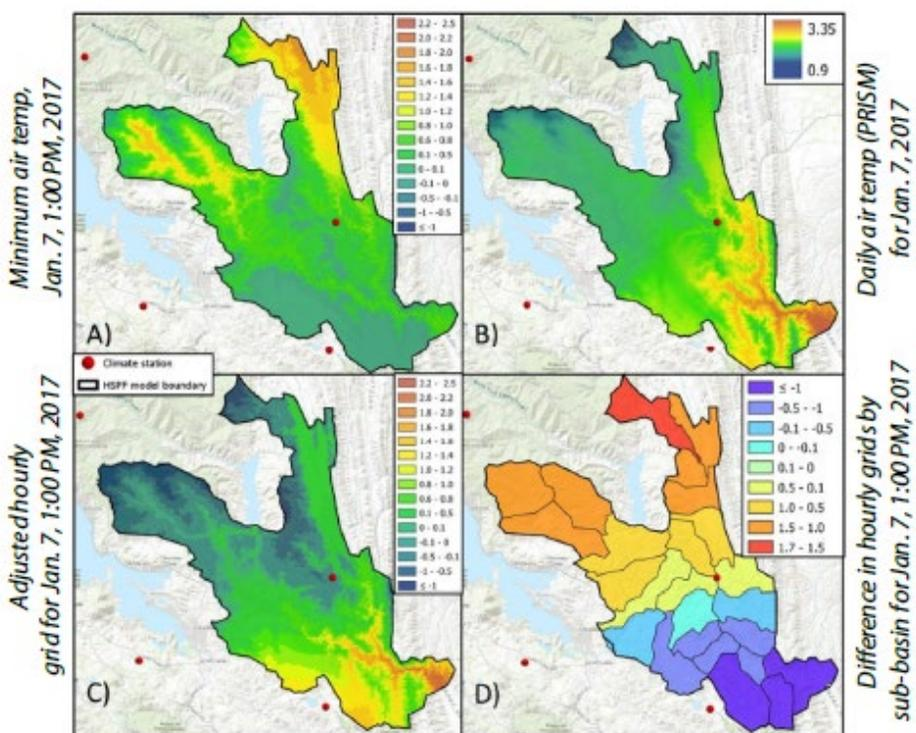
Fig. 8: Interpolation steps from hourly station data to gridded weather grids for Cache Creek, CA.
